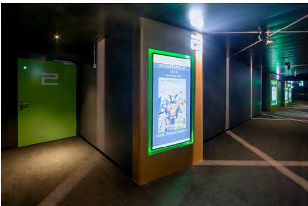
Here the lighting is kept deliberately low-key to allow the illuminated advertising boards to stand out. Pools of light are created in the service areas by recessed downlights set behind a stretched metal ceiling, while backlit stretched ceilings serve to define the seating areas. The walls are defined by uplighting, forming a strong focal point, along with the brighter lighting in the cashier areas.
