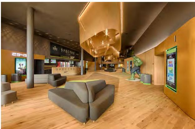
The more prominent feature is created with a metal mesh curtain. For this piece, two lighting components simultaneously create the transparent volume and enhance the brilliance of the material. Firstly perimeter lighting LED fittings take care of general lighting while defining the material from different viewpoints. Secondly, internally suspended unshielded miniature LED bulbs mounted at different heights transform the feature into a unique modern chandelier.
